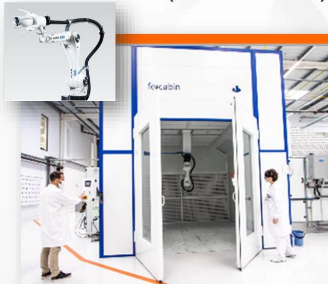
PAINT BOX WITH SPRAY ROBOT KUKA READY2SPRAY (SPRAYHEAD DÜRR)
