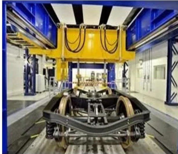
World's first carbon fiber rail bogie (Source: Materials Today: Proceedings)
