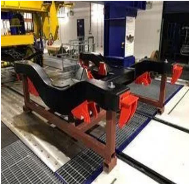
World's first carbon fiber rail bogie (Source: Materials Today: Proceedings)
